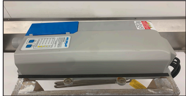
12. The EECA cover should be flush with the center module.
