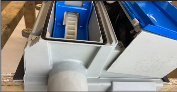
11. With the skimming wheel cover open, place the new EECA on the center module.
