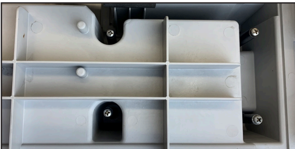
13. Close the flip door cover and flip the center module. There will be (4) bolts in the front and (1) on the rear.
