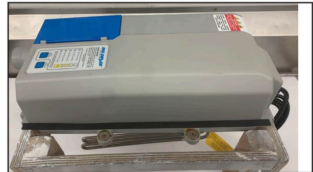
16. EECA cover should be flush with the center module.
