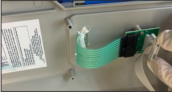
5. Disconnect the push button ribbon from the push button adapter.
