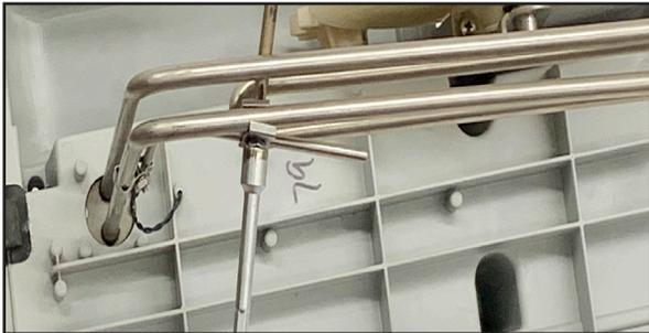
7. Turn the center module upside down. Use a Phillips head screwdriver and a 5/16 nut driver to remove the (2) secured clamps holding the thermistor. Set the clamps aside.
