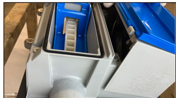
4. Lift the cover over the skimming wheel to pry open the EECA cover. Pull upwards until EECA is completely removed from the center module.
