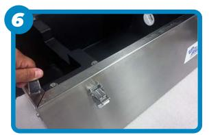
Repeat this process with all sides until the gasket is removed. Some residue may remain.
