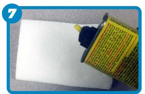
Remove remaining residue with an adhesive remover and a clean rag. Acetone works best.
