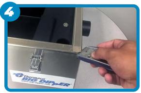
Remove the gasket by using a razor blade, paint scraper, or other sharp item.
