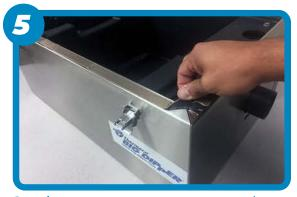
Starting at one corner, remove gasket by slowly pulling upwards and scraping residue with blade.
