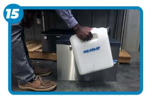
Place grease collector on unit by lining up the grease collector with the opening on the unit. Turn the collector slightly clockwise to lock into position.
