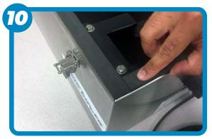
Repeat measuring and placing new gasket on the back, then sides of tank. Do NOT overlap
