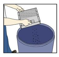
2. Check grease collector and empty if needed
