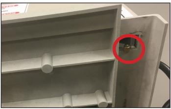
2. Locate safety switch on the bottom portion of the Electronic Assembly.
