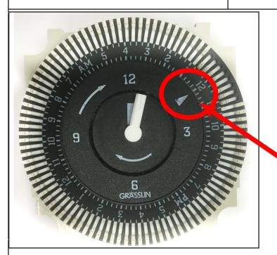
1. Big Dipper units 14000 series or earlier are controlled by a timer. To begin troubleshoot, locate the time of day arrow on the timer and rotate the timer to be set on 12 as illustrated. (Please note, to have the unit in the ON position, push tabs towards the middle on the time of day arrow.)
