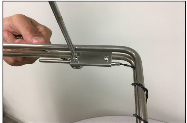
10. Wrap Thermistor wire around heater and secure Thermistor by installing both screws and bolts used to remove.
