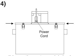
4) Lower the center module back down on top of the unit. Move the two side wings back into place & fasten all six latches.
