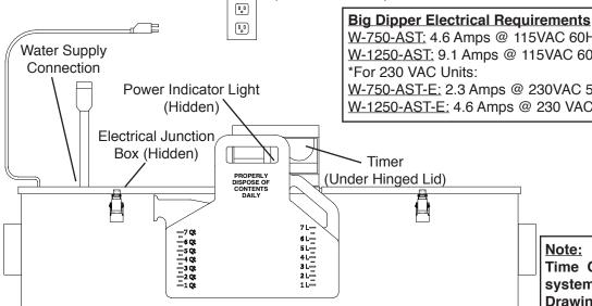
W-750-AST: 4.6 Amps @ 115VAC 60Hz (535 Watts) W-1250-AST: 9.1 Amps @ 115VAC 60Hz (1055 Watts)
