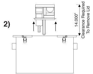
2) Lift the center module up off of the unit, ensuring clearance for the heater.
