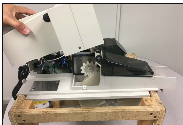
22. Replace the front and rear enclosure covers and secure with (2) screws in the front enclosure, (2) on each side and (4) on the rear enclosure.
