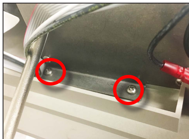
16. Place board on Electrical Assembly and reuse (2) screws to secure board on Electrical Assembly.
