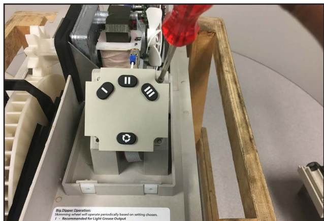
21. Install Push Button Interface Board and reuse (2) screws to secure board.
