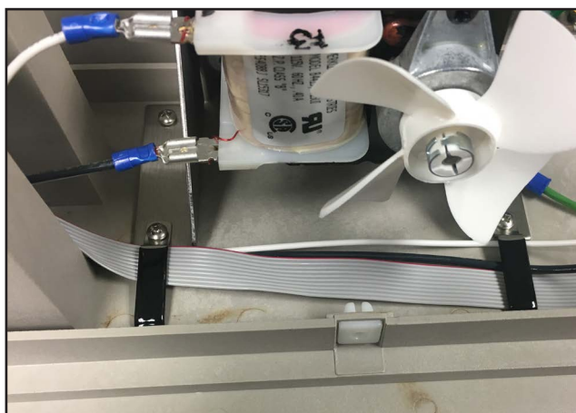
15. Install new ribbon under plastic strip and secure each strip with screw.
