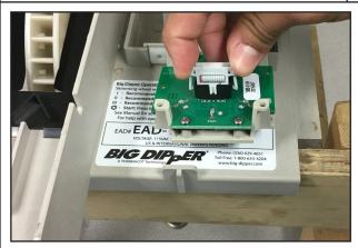
7. Pull outer tabs out and disconnect ribbon from Push Button Interface Board.
