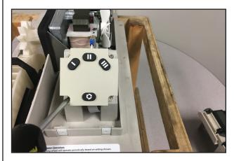
5. Locate the Push Button Interface Board and remove (2) screws.
