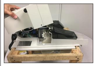
3. Lift cover up and remove rear enclosure.
