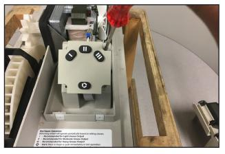
8. Install new Push Button Interface Board and Replace the (2) screws used to remove the Push Button Interface Board.
