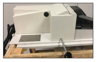
2. Remove (2) screws from the front enclosure,(2) on each side and (4) from the rear enclosure.
