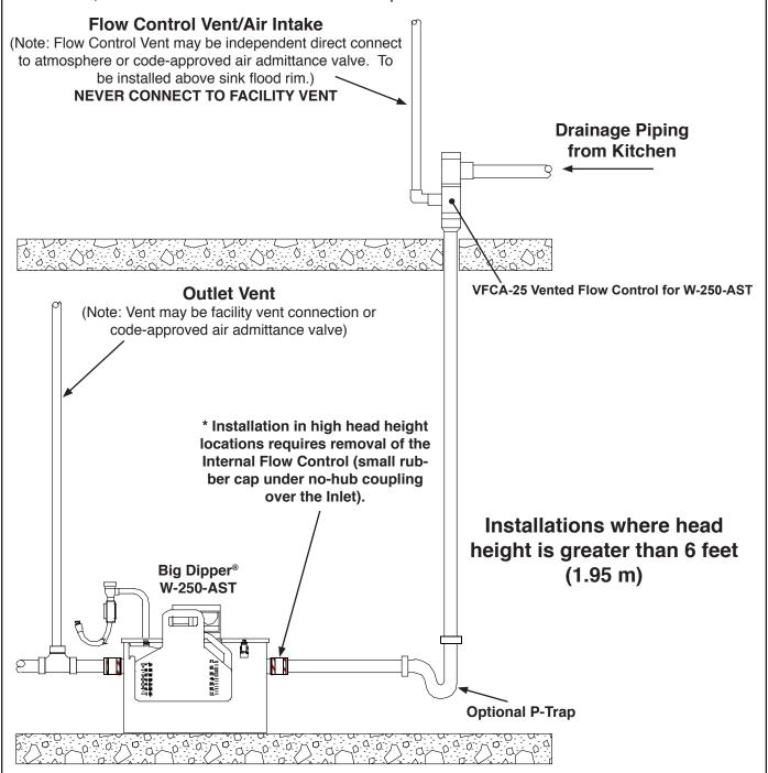
NOTE: Drawing for reference only. Equipment must be installed in compliance with all applicable laws, requlations and codes, including plumbing codes. Installation should be performed by a qualified plumber.
