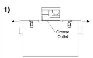
1) Unlatch the Unit lid. Pull the side wings outward.
